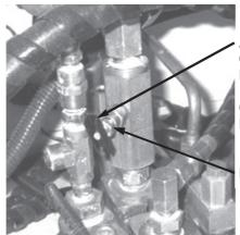
ADJUSTABLE NEEDLE: COUNTERCLOCKWISE = FASTER LOWERING SPEED
